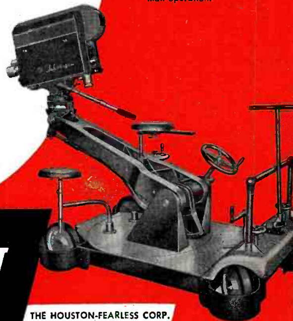
H-F Panoram Dolly provides countless camera effects . . . raising, lowering, panning, tilting, and dollying. Smooth and steady.
